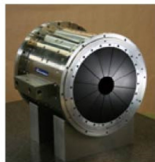
6極磁気回路完成写真 Overview of 6-pole magnetic circuit
